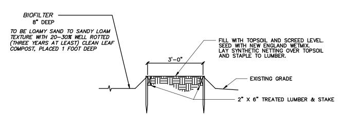
SEED BIOFILTER AND LEVEL SPREADER WITH NEW ENGLAND WETMIX AT A RATE OF 1 LB./2500 SQUARE FEET.
