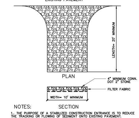
3. THE ENTRANCE SHOULD BE MAINTAINED IN A CONDITION WHICH WILL PREVENT TRACKING OR FLOWING OF SEDIMENT ONTO EXISTING PAVEMENT. THIS WILL REQUIRE PERIODIC TOP DRESSING WITH ADITIONAL STONE OR ADDITIONAL LENGTH AS CONDITIONS DEMAND.
